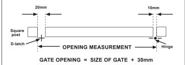
**Step 2** - Fix the butt hinges to the gate first. Tek screw these on at approximately 100mm from the top and 100mm from the bottom. It is recommended that the hinges be face mounted. Use the stainless steel tek screws supplied.
